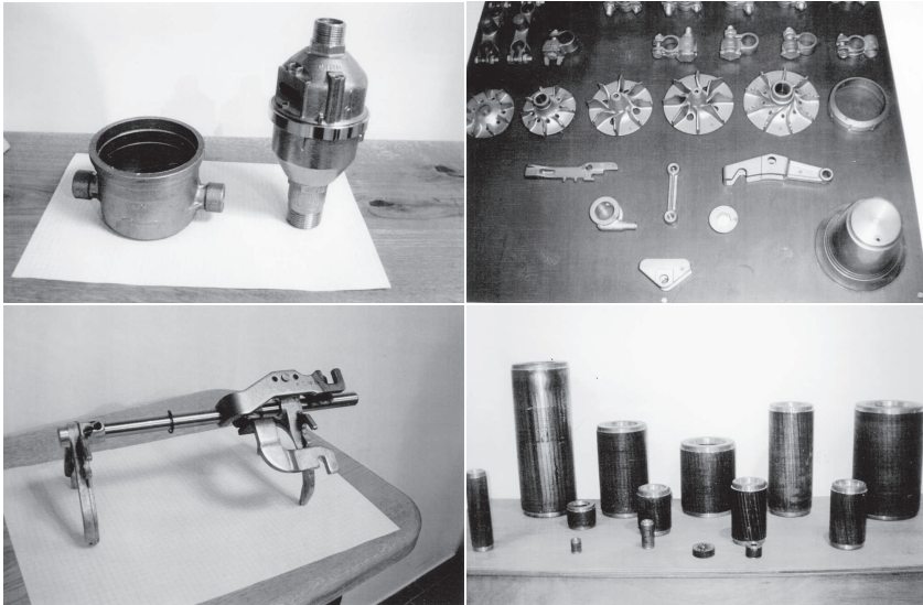
Figure 4-1. FAVI's changes of business since 1950: sanitary siphons for sink drains (top left photo), water gauges (top right), automobile shift forks (bottom left), electrical generator rotors (bottom right). (Figure created by French quality expert Martine Morel.)
